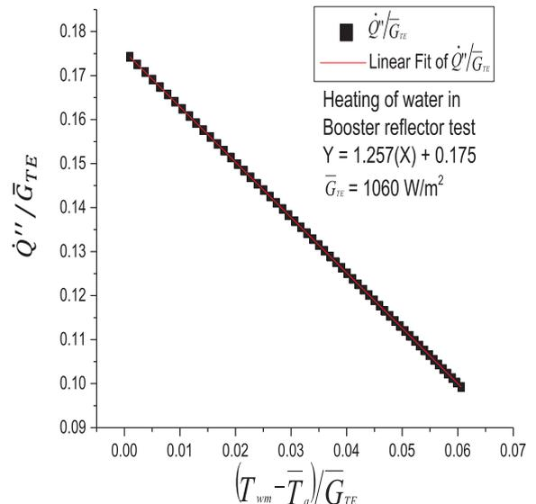
Fig. 4b. Plot of  $\frac{\dot{Q}''}{\bar{G}_{TE}}$  with  $\frac{(T_{wm} - T_a)}{\bar{G}_{TE}}$ .
