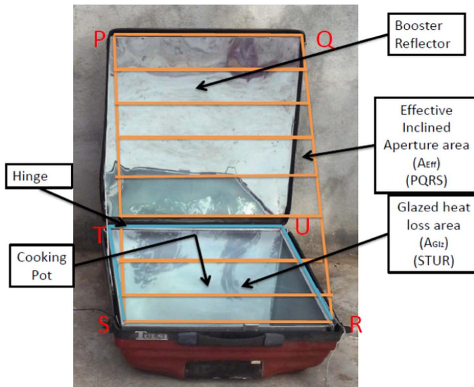
Fig. 1. Inclined aperture area ( $A_{Eff}$ ) and the glazed heat loss area ( $A_{Giz}$ ) for a specified SBC.
