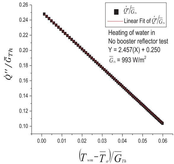
Fig. 3b. Plot of  $\frac{\dot{Q}''}{\bar{G}_{Th}}$  with  $\frac{(T_{wm} - T_a)}{\bar{G}_{Th}}$ .
