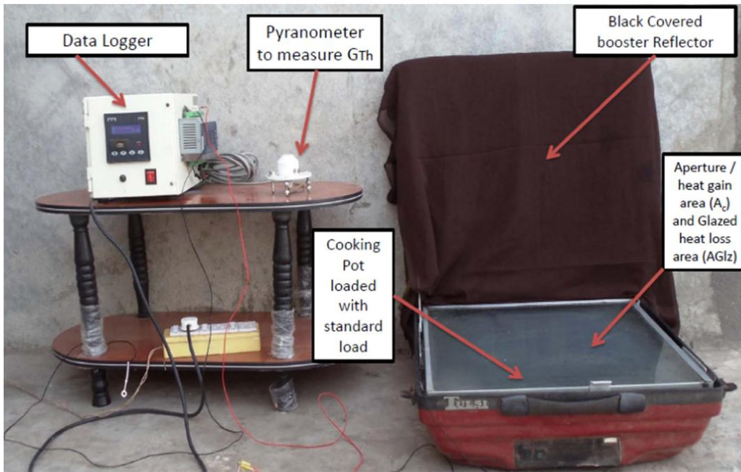
Fig. 2a. Test set up for No Booster Reflector Test.
