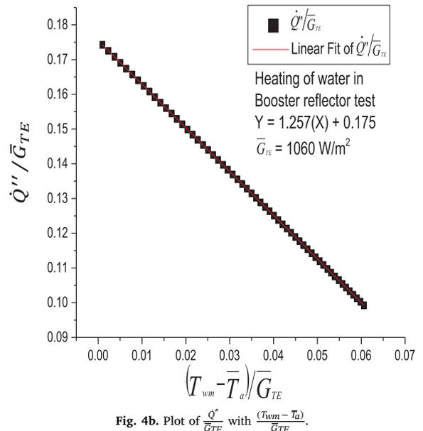
Fig. 4b. Plot of  $\frac{\dot{Q}''}{\bar{G}_{TE}}$  with  $\frac{(T_{wm} - T_a)}{\bar{G}_{TE}}$ .
