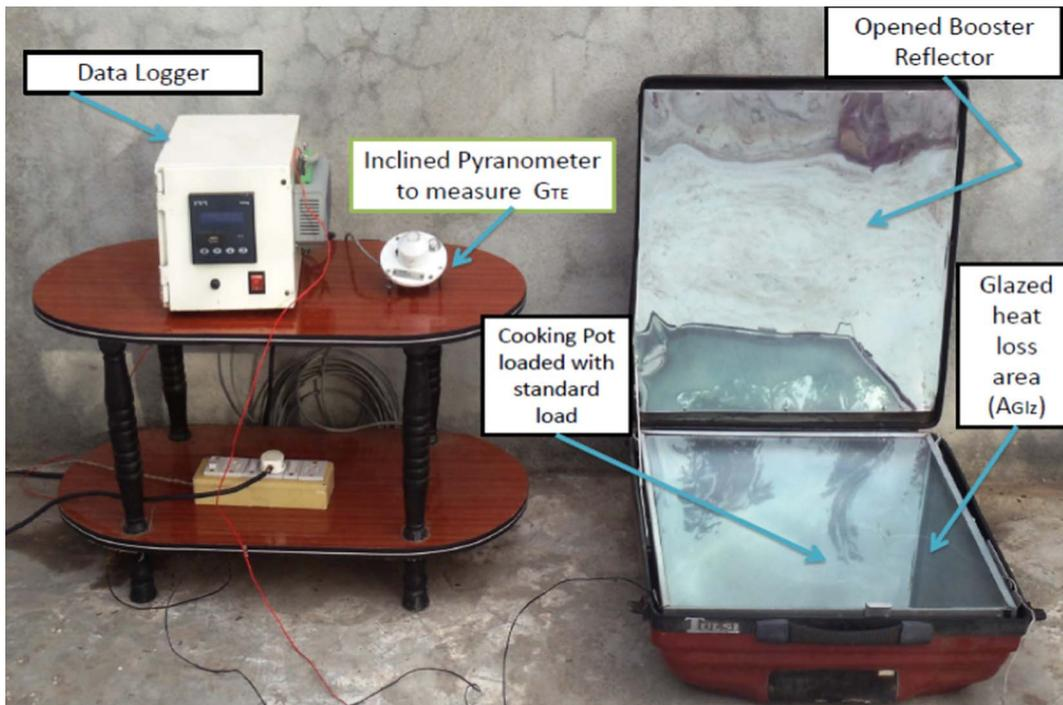
Fig. 2b. Test set up for a Booster Reflector Test.
