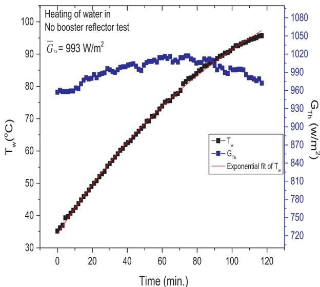
Fig. 3a. Variation of water temperature with time for no booster reflector test.
