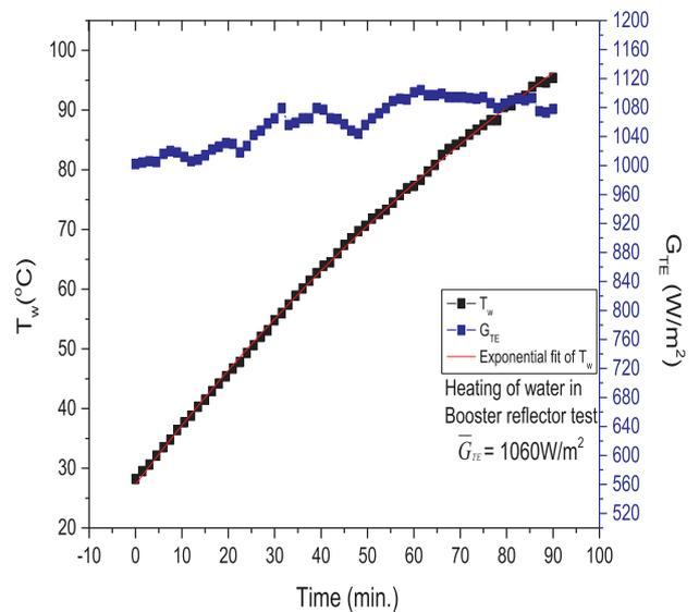
Fig. 4a. Variation of the water temperature with time for booster reflector test.
