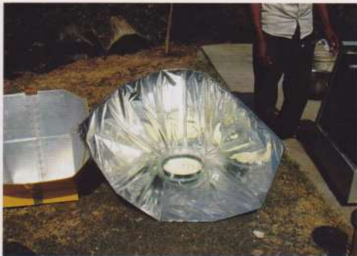
A collapsible solar cooker that can be folded up and taken any place under the sun for cooking a meal
