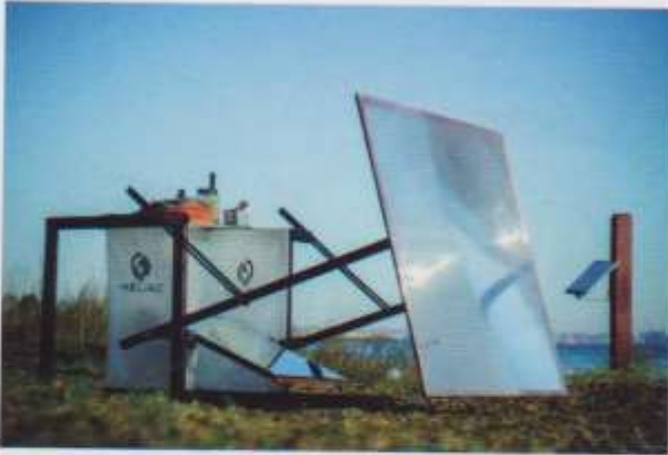
Heliac, of Denmark, has created a prototype of concentrator solar cooker made with special solar concentrating foil
