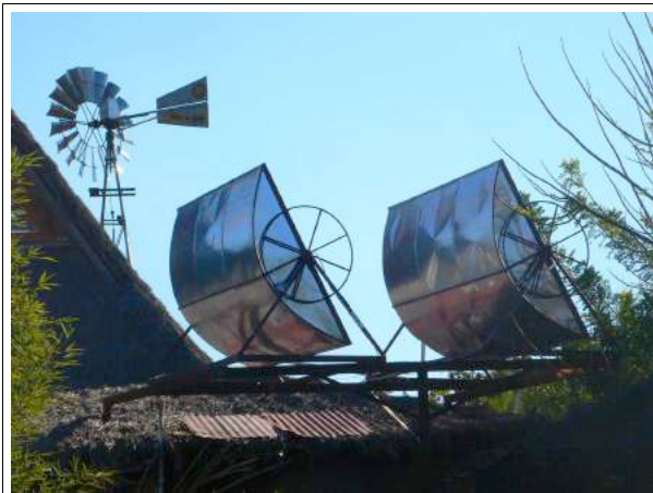
Picture 6: The reflectors of the gastronomy steamer.
