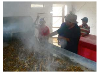
Picture 10: Opening the steaming drum distributing the corn straw on the table.
