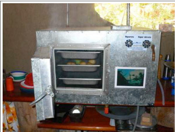
Picture 7: The steaming compartment.
