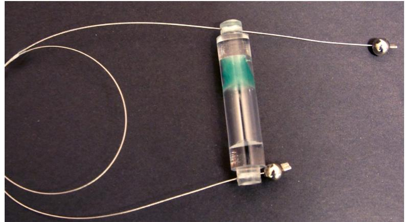
**The SUPERWAPI** can be used both with a solar oven and when the sun isn't shining or at night. The Super WAPI features a stainless steel cable that is highly resistant to heat and can be used with solar or fossil fueled heat. It saves almost 50% on fuel (and thus cost) because the water has to reach only 149° F to be pasteurized. It makes water safe from microbes like e coli, rotaviruses, giardia and hepatitis A.
