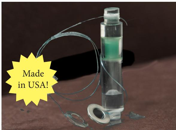
**The Cool WAPI** has a nylon cord that drapes over the edge of the water pot to allow the operator to lift it from the pot without scalding fingers from the hot water. Stainless steel washers are tied to both ends of the cord to weight down the Cool WAPI. The operator can lift the Cool WAPI from the water to view the wax condition, and invert to relocate the wax at the top of the tube, allowing for unlimited reuse.
