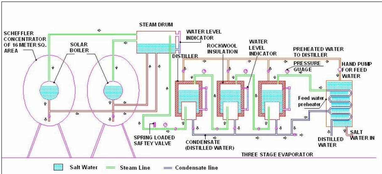
Fig. 4.1 Schematic layout of Multistage evaporators with Scheffler concentrators & H.R. unit.
