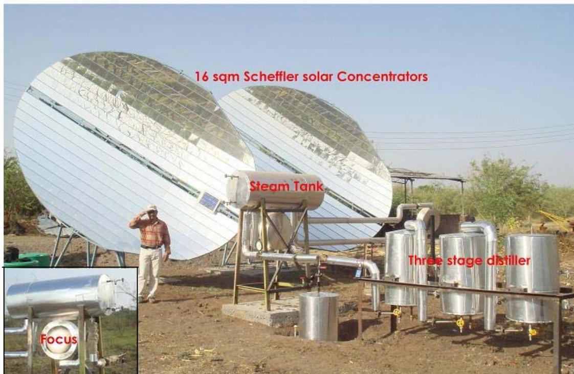
Fig. 4.2 : Photograph of Solar steam generator with multistage evaporators.
