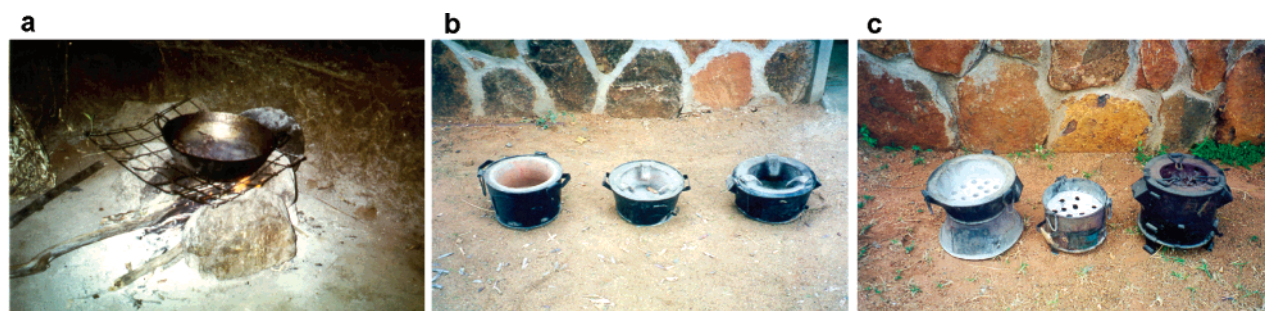
FIGURE 1. Stoves used in the study area. (a) Three-stone fire with metal grate. (b) Ceramic-lined woodstoves (from left to right): the Upesi, the Kuni Mbili, and the Lira. (c) Charcoal stoves (from left to right): the Kenyan ceramic Jiko (KCJ), a single-walled metal stove, and a double-walled metal stove (Loketo).
