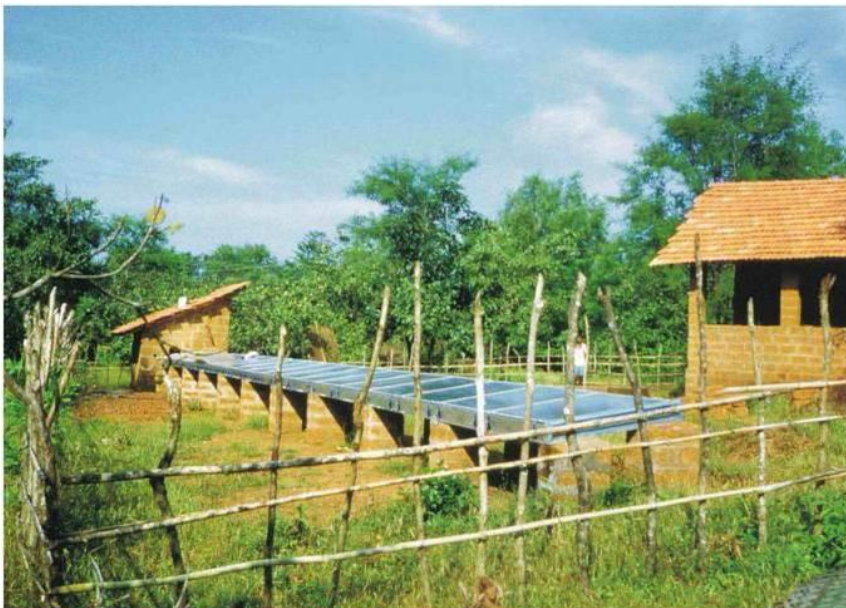
Picture 1 shows a tunnel dryer for drying food with solar energy developed at the Technical University of Munich (German-Indian Solar Drying Project)
