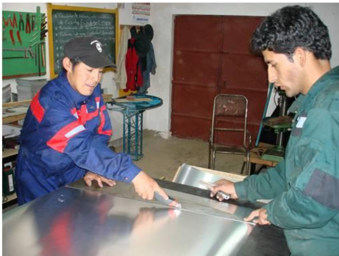
Picture 2 shows the cutting of high-gloss aluminum sheets in a workshop in Bolivia for the production of parabolic solar cookers of SK design.
