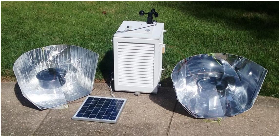
Notice that there are two solar cookers under test. Two or more items may be measured at one time in order to check repeatability and increase productivity. This system can actually measure up to four cookers at one time. (The test platforms were not constructed at the time of this photo.)
