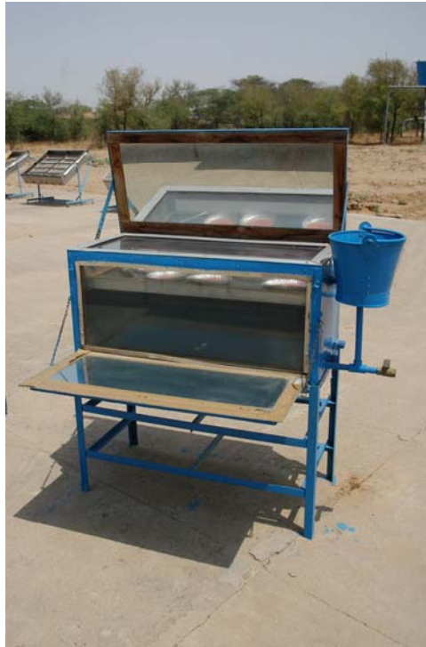
Fig. 1. Drying of watermelon crush in the integrated device designed and developed at CAZRI, Jodhpur
