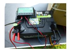
Here are some images of the cooker in action. On the left you can see the solar panel and the solar box oven facing the sun. The middle image shows the heating pad. Later experimentation showed that it worked better when in contact with the pan. The right hand side image shows the battery with the charge controller stuck on top. The terminals are insulated to prevent accidental shorting and there is a 10 Amp fuse in series with the positive terminal of the battery.
