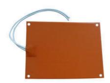
The first task was to find a suitable heating element and was surprised to find one quickly on E-Bay. It was priced at £15 (\$22). All one had to do was to connect it directly to a 12V supply and it was waterproof — an essential requirement inside a cooker. In air they will settle at a temperature of approx 160 to 170C. The waterproof covering can handle a maximum temperature of approx 220C.
