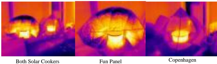
Figure 1. Thermal image of Fun Panel on left and Copenhagen Solar Cooker on right.
