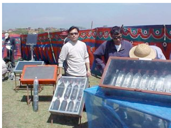
Fig.3 Water Pasteurizers - different types made by FoST
