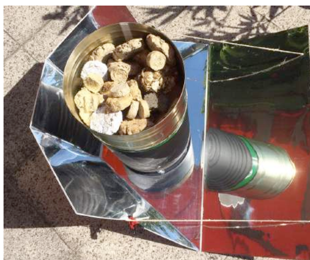
Photo 7 (right): The dryer for solar panel cookers is mainly designed as a food processing unit for fruits and vegetables.
