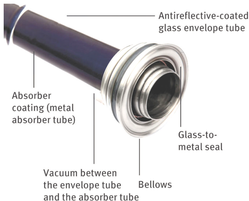
Figure 2. A metal in glass absorber tube manufactured by Schott AG [13]
