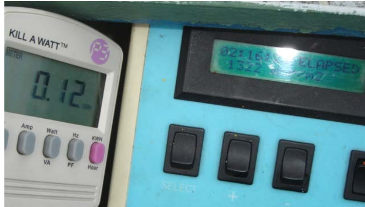
Photo 8. Measurement of integrated electric (left) and solar (right) energy used.
