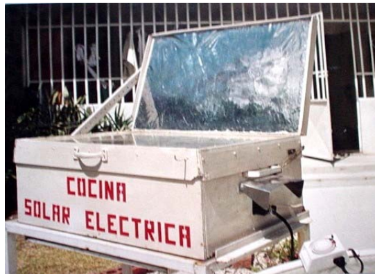
Photo 2. Hybrid Solar Oven with 110 VAC Electricity and Sun (1986).
