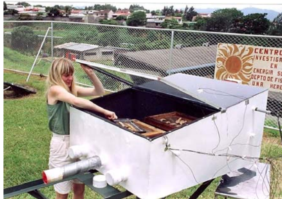
Photo 3. Natural and forced circulation Solar Dryer (1994)
