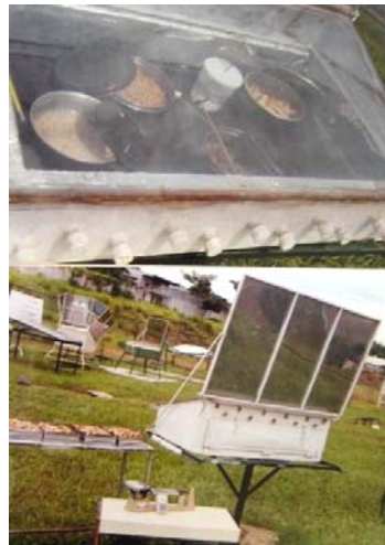
Photo 6. Passive Cooker cum Dryer (1993).
