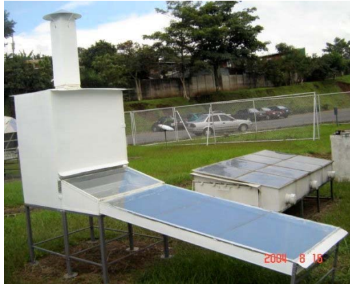
Photo 5. Direct and Indirect Solar Dryer (2007).
