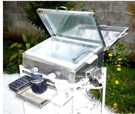
Photo 7. Hybrid Fuel Food processor (2005): 1. Electric plate, 2. Electric inlet and thermostat, 3. Reflector, 3A. Rod to adjust reflector, 4. Two inlet holes for air, 5. three outlet holes for humid air, 6. Outer box, 7. Electric Timer, 8. bottle for distilled water, 13. Trough/ gutter for distilled water.
