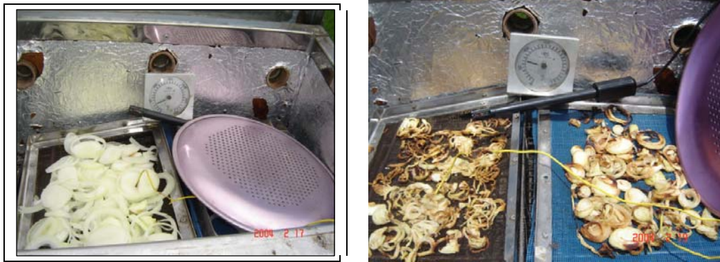
Photo 10. Food processor in the mode of drying, fresh (left) and dried (right) onions.
