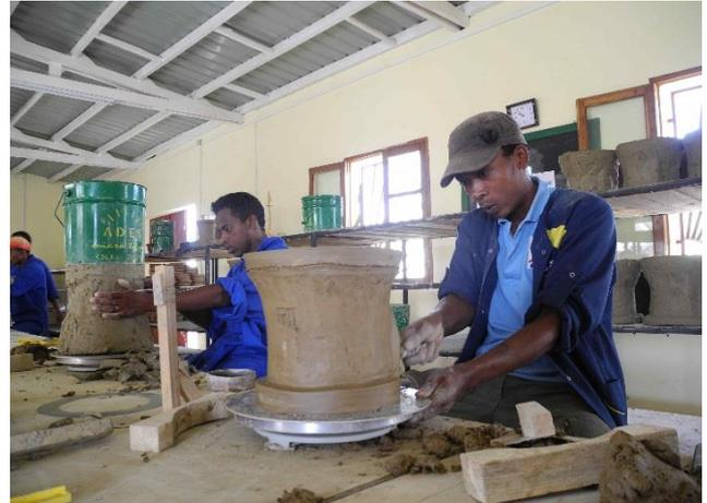
*processing of clay cores for energy-saving cookers*
