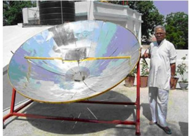
**Photograph 1: Dr. P.T. Joshi with 2.3 m dia. Parabolic dish concentrator, preparing ayurvedic syrups.**
