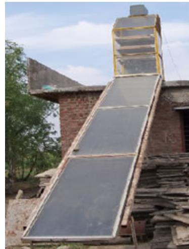
**Photograph 4: Low cost solar dryer for agro processing.**
