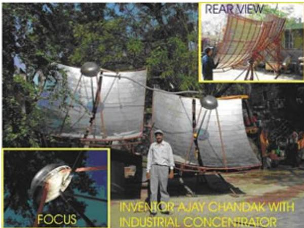
**Photograph 2: 'Industrial Solar Concentrator' for hot air up to 200°C**
