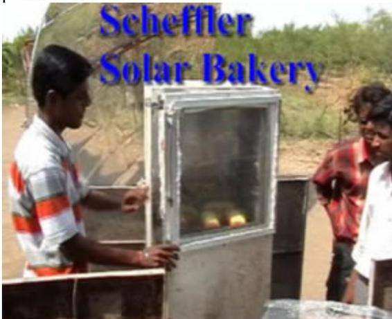
**Photograph 3: Oven used for bakery using Scheffler Concentrator.**
