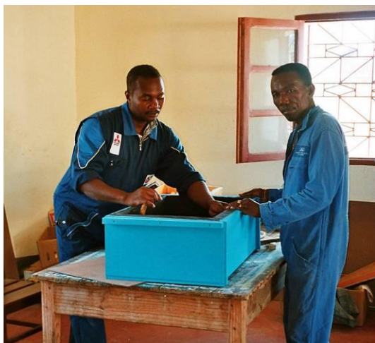
ADES carpenters fabricating box solar cookers
