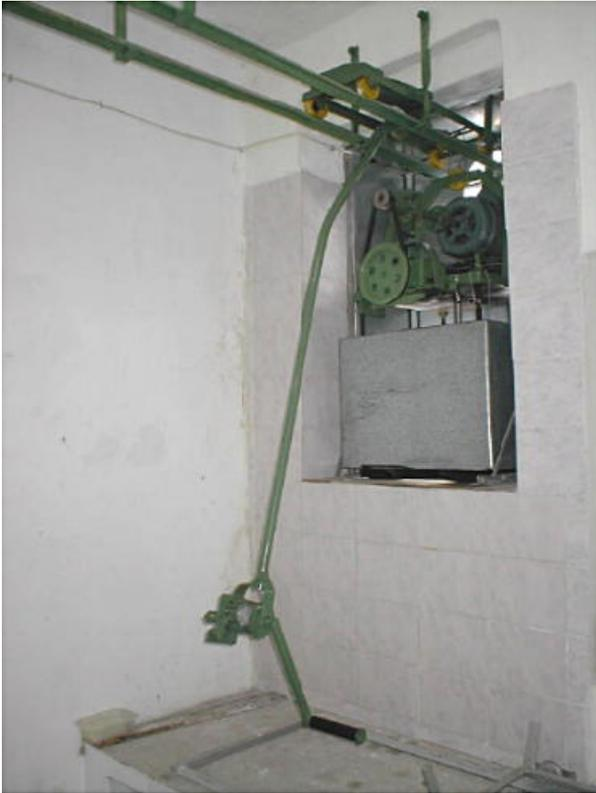
**Fig. 4. Cooking pot in cooking position (with insulating panels) and elevating system**
