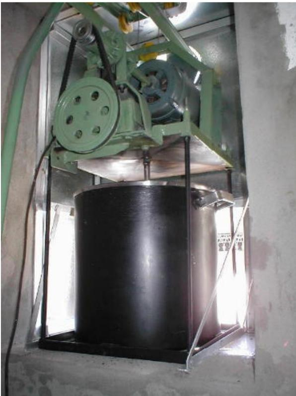
**Fig. 3. Cooking pot inside its cage with mixer put on the cooking place (without insulating panels)**
