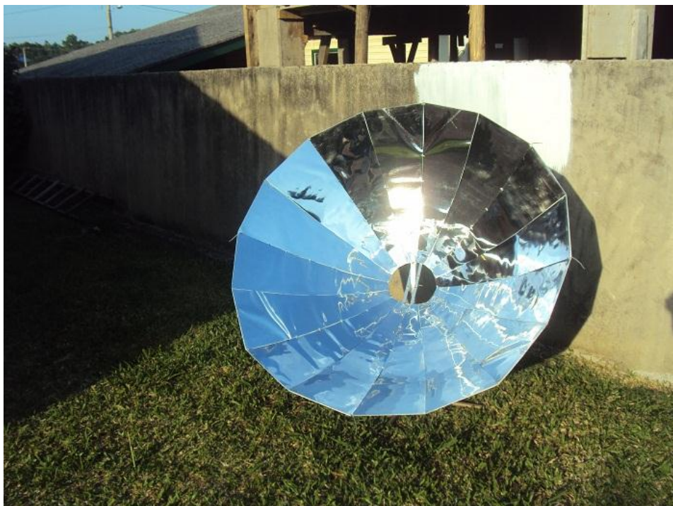
Fig 3 – A 16 petals 1.2 m diameter parabolic SC with Coroplast and Mylar glued
