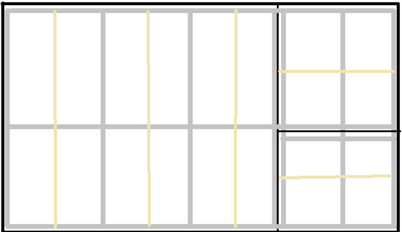
Fig 5 – Fun Panel SC side with double sided tape (gray) and glue line (ambar)
