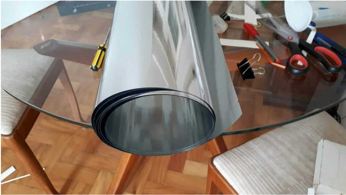
Fig 8 – Low cost no adhesive Mylar roll reflective film – thickness of .25 mm
