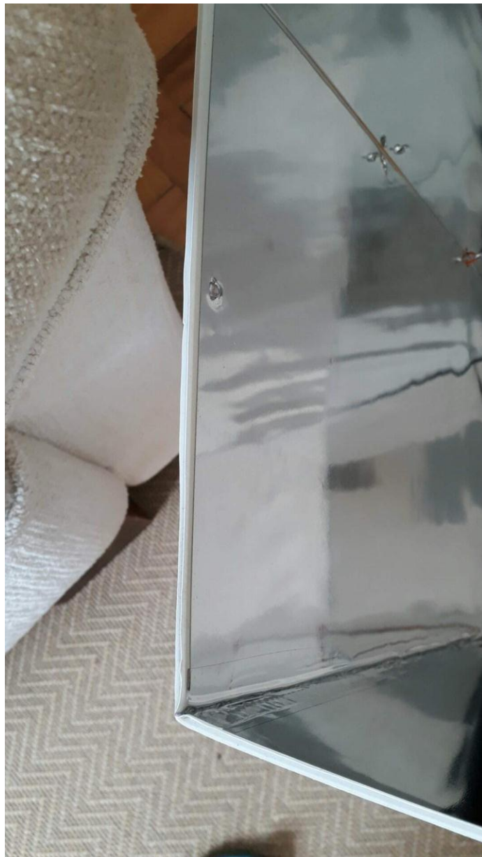
Fig 9 – Detail of a Fun Panel SC with Coroplast glued with Mylar
