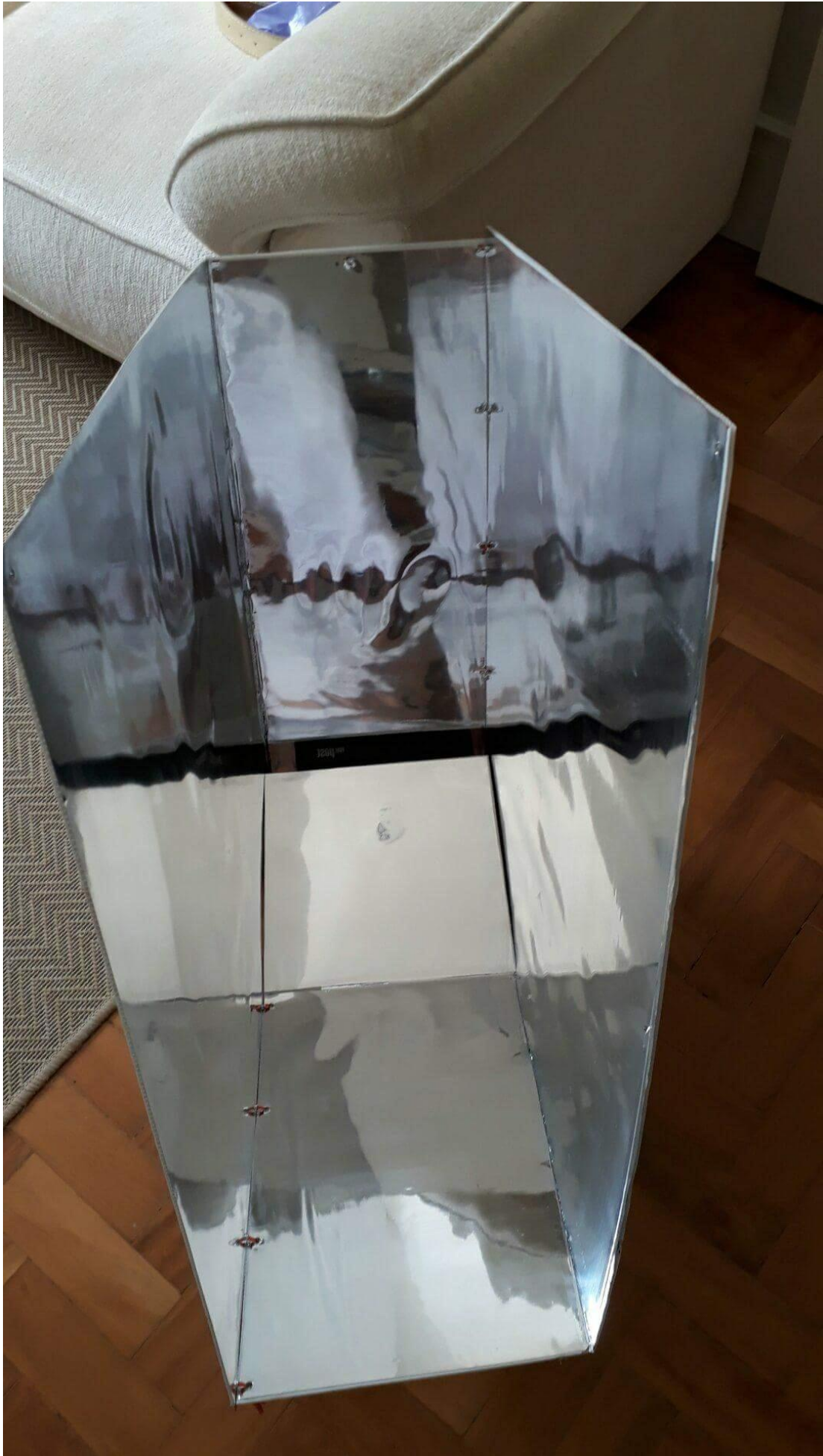
Fig 10 – Detail of a Jumbo Fun Panel SC with Coroplast and Mylar. Must be opened with ties
