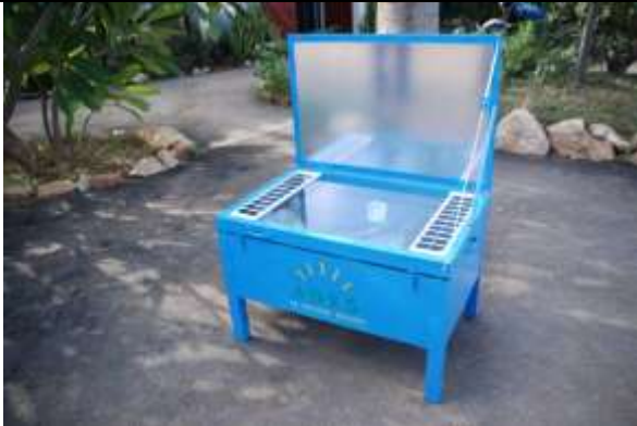
Box-type solar cooker with integrated electric charger
