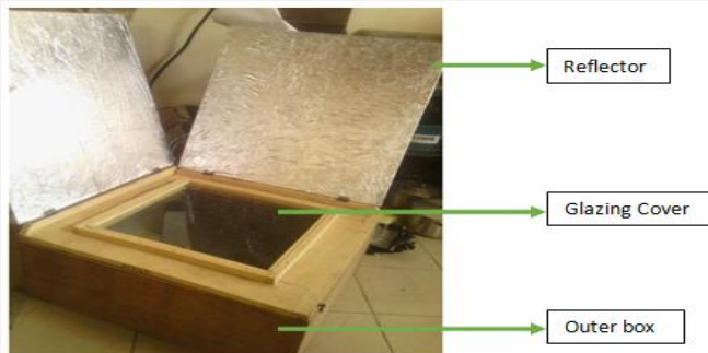
Figure 1: The Constructed Solar Box Cooker
