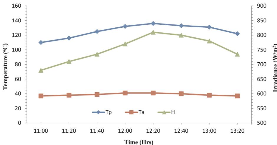
Fig. 4. Stagnation testing of new SBC on configuration 1.
