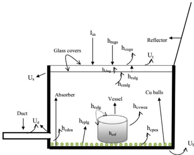
Fig. 3. Heat transfer mechanism of solar cooker.
