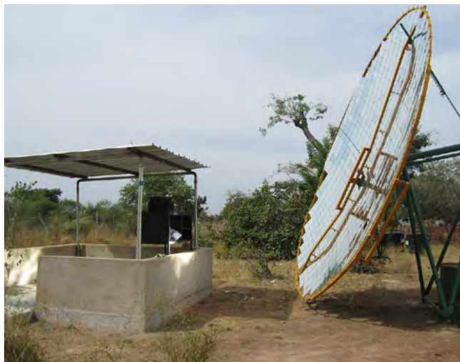
Fig. 3. Set up Scheffler reflectors for community kitchens.
