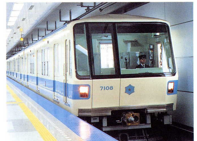
Intermediate Capacity Rail System - System with an hourly capacity of 20,000 to 40,000 passengers per direction, compared to 50,000 to 75,000 for MTR
